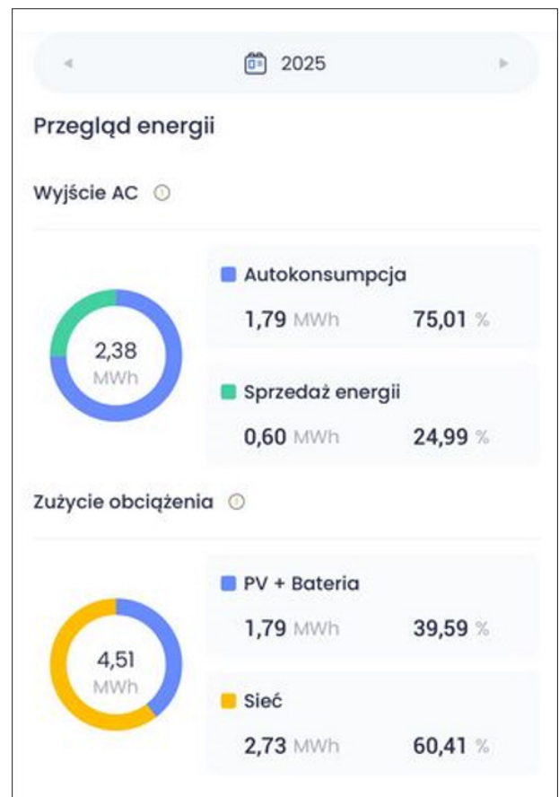
Fot. 2. System PV 28 kWp bez BESS
